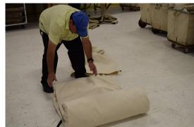
**Step 8:** Position Tent along sided of frame top and pull over top of frame
