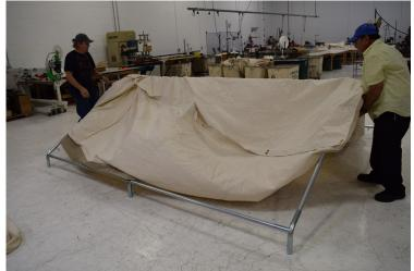
**Step 8:** Open Ridge Pole zipper and insert eyebolts through tent grommet at each end peak.
