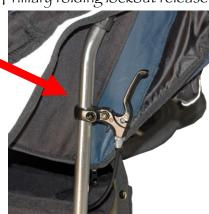
Squeeze and hold the lever, while pushing down slightly on the AXIOM handle. Once the AXIOM has started to fold, you may release the lever.
