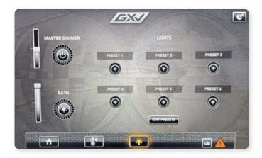
NOTE: You can only edit the Preset currently highlighted on the display. Select the desired Preset, adjust the light settings and hit Save.
