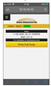
This is useful when the fuel line to the furnace sucked air due to maintenance or an empty fuel tank and the line needs priming. When tapping this button, the fuel pump will activate the 5S. Do NOT use this function unless directed by a technician.
