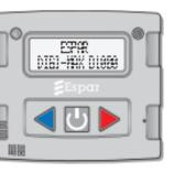
3b. If you want to clear the fault codes, press the Red button for Yes. The next screen will confirm the ECU reset, followed by a screen, which will give you the option to check for codes. After clearing codes, the code reader will cycle back to the default screen and return to normal.
