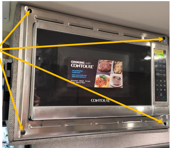
Figure 14 Remove (4) screws from microwave trim
