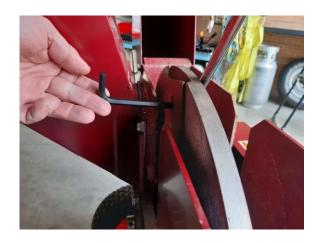
In order to fully remove the nut and bolt, use an 8mm Allen key to counter the force from the spanner. Remove the nuts and bolts from the chipper blade. Once all three have been removed, take out the chipper blade.
