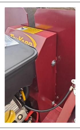
Remove the protective cover that sits over the belts with a 13mm socket.
