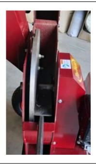
Open the discharge chute and place a bar between one of the flaps of the flywheel and the frame of the machine as shown. Ensure that the flywheel doesn't rotate when this bar is in place by pulling the engine cord.
