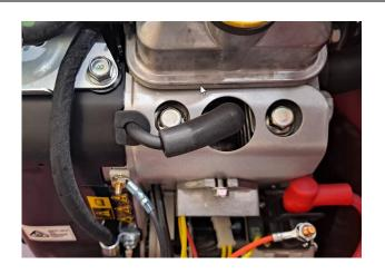
Disconnect the spark plug to ensure that the machine will not receive power whilst you are working on the flywheel
