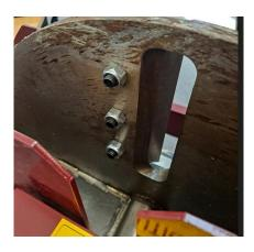
Using a 19mm spanner, loosen the nut and bolt that connects the chipper blade to the flywheel.
