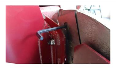
When retightening the nut and bolt, the rotation of the spanner will force the flywheel the opposite direction. Use the Allen key against the frame of the machine as pictured to prevent the flywheel from rotating whilst the nut is being tightened.
