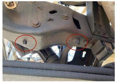
11. The sway bar brackets are tilted in towards the frame and back towards the axle.
