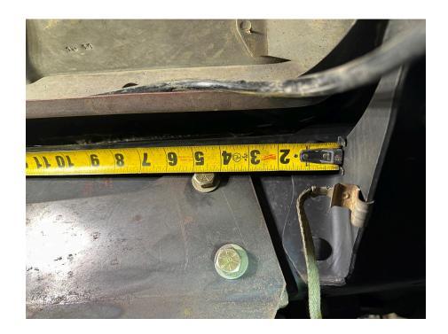
(4WD) For reference the top bolt hole will be 4 ½" from the body mount to the center of the bolt hole. Once you have confirmed that everything lines up, align the BDD brackets to the obs frame using clamps to hold in place while you install or enlarge the existing holes. Once you have the bolts installed, snug up the bottom holes to the bracket until the bracket is snug onto the frame. Then tighten the bolts located on the side of the frame.
