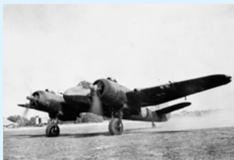
A Bristol Beaufigther, with “arrowhead”, folded twin-dipole antenna on the nose for its VHF-band AI radar
