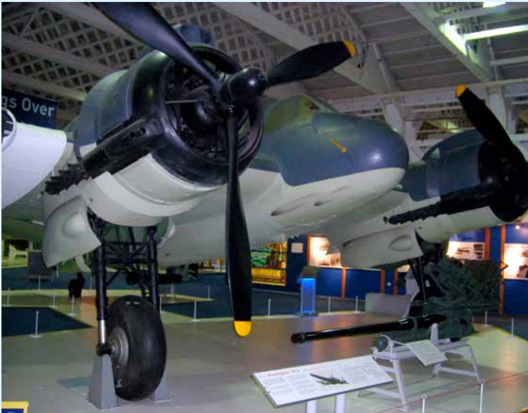
Bristol Beaufighter TF X RD253, at the Royal Air Force Museum London. On the floor below is a 6-pounder gun with Molins autoloader, as mounted on the de Havilland Mosquito “Tsetse”
