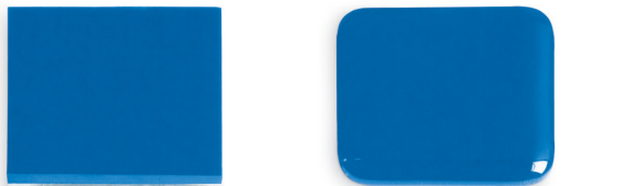
Figure 1: Two, 1/8" (3 mm) layers fired to 1500°F (816°C). Notice that the area covered stays the same and the edges are straight.
