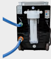
Chiller and Water Filter Housing
