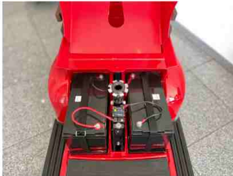
Figure 7: Batteries and battery connections
