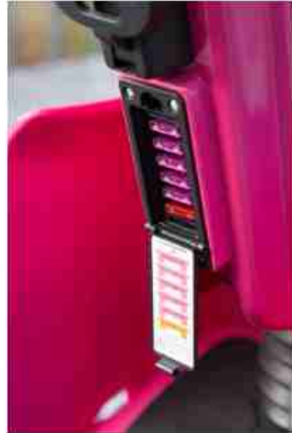
Figure 9: Electrical system fuses
