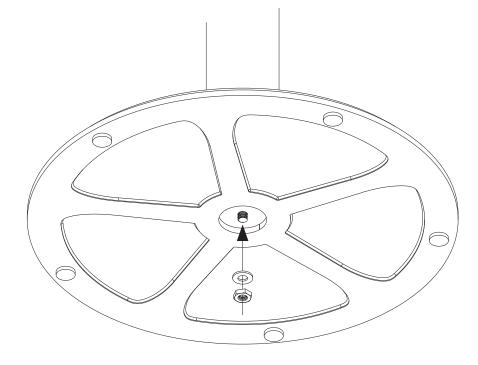
Using the spanner, tighten down the bolt and washer. This connection must be very secure to prevent wobbling.
