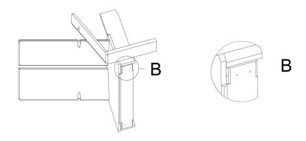
3. Next, return the assembled parts upright and insert the second arm. Use  $2 \times 10^{-2}$  x screws on the armrest joints.
