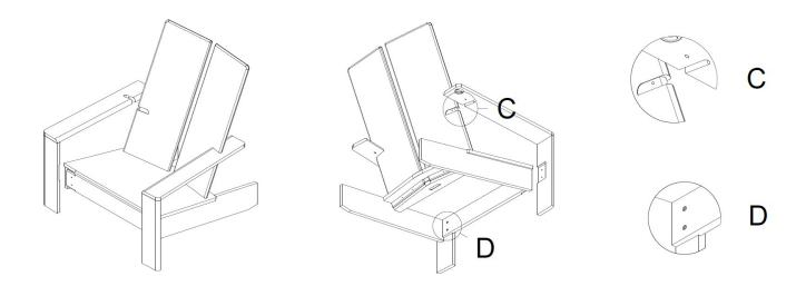
${\bf 4}.$  Once all parts are assembled, bolts can be tightened further.
