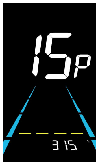
Figure 6-15 Battery under voltage value setting interface
