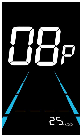
Figure 6-8 Speed limit setting interface
