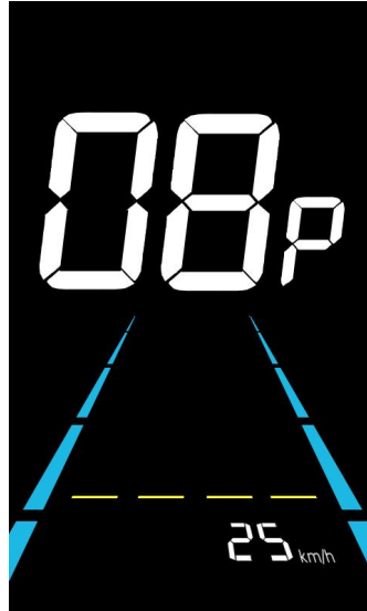
Figure 6-8 Speed limit setting interface
