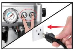
**O3.** Once plugged it in, release the Single and Double buttons and press the HOT WATER button immediately.
