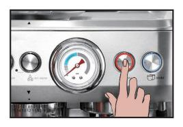
**O7.** The Single button will start flashing in red, and the Double button turns off, which means that the machine is in the process of initializing the program.
