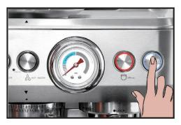
06. The Double button will start flashing in red, and the Single button turns off, which means that the machine in the process of correcting the program.
