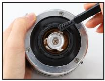
O6. Clean the inside of grinder with the cleaning brush.
