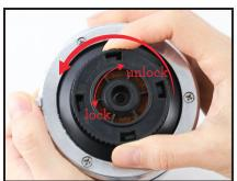
O9. Note: The fastener of distributor must point at the groove of grinder. Otherwise, the distributor could not be assembled successfully.
