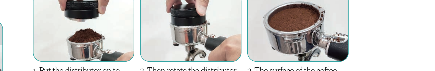
1. Put the distributor on to the portafilter. 2. Then rotate the distributor to even the surface of coffee grounds. 3. The surface of the coffee grounds is now even, but the inside of the coffee grounds is still loose.
