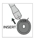
**04.** If the hole of the steam wand remains blocked. Unscrew the steam nozzle and put it into a cup of warm water with one espresso machine cleaning tablet. Rinse the steam nozzle under running water, then insert the cleaning needle into the hole and remove. Run hot water through the steam wand for 4-6 seconds.
