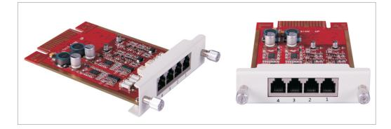
2FXOS (Foreign Exchange Office & Foreign Exchange Station) 2FXOS is mixed interface of foreign exchange office and foreign exchange station that connect to office and station. It includes 2FXO ports and 2FXS ports, and can be combined with BRI, PRI, GSM module.
