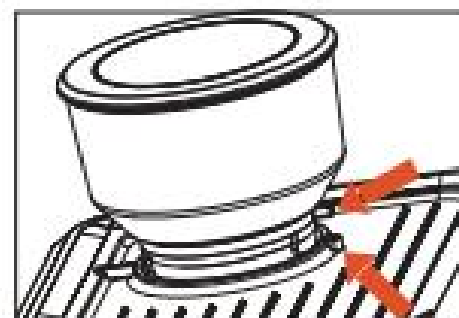
Figure 2: align the positions in red circles in the figure, and press it down, rotate it clockwise and install it into the machine.
