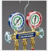
Forged body is solid brass for durability. Full porting maximizes capacity. Metal valve handles are full size for easy operation. Hose anchors are forged into back of body at 45°.
