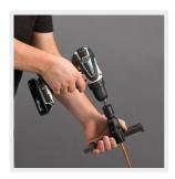
The aluminum body of the YELLOW JACKET Crimping tool is only half as heavy as conventional steel structures. For superfast beading, remove the upper handle and replace it with an electric drill drive.
