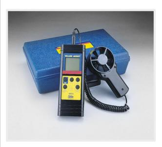
This hand-held instrument reads both air velocity and temperature simultaneously when balancing air conditioning/heating ventilation systems.
