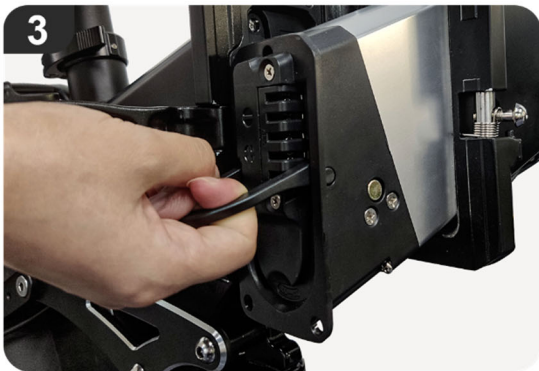
3. Fold the frame and remove the battery.
