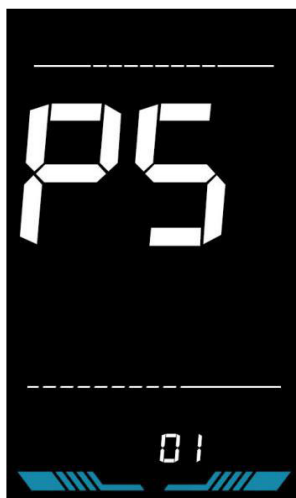
Figure 6-6 Number of speed sensor magnets setting interface
