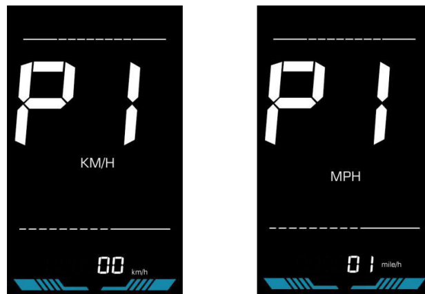
Figure 6-1 Metric and Imperial Units Setting Interface
