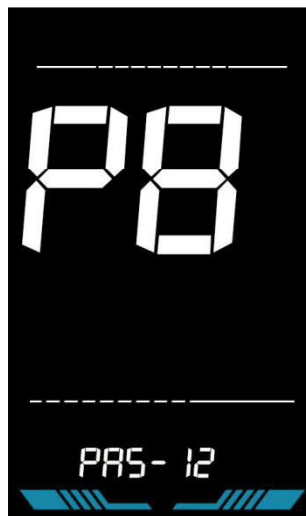
Figure 6-11 Pedal assist sensor magnets setting
