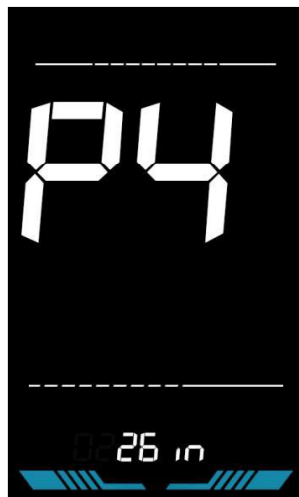
Figure 6-5 Wheel diameter setting interface
