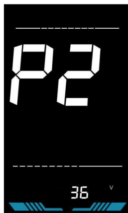
Figure 6-2 Rated voltage setting interface
