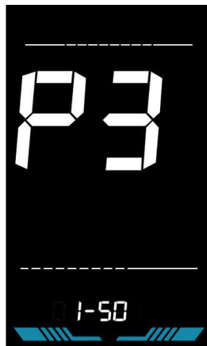
Figure 6-4 PAS level ratio value setting interface
