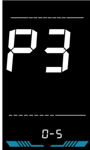
Figure 6-3 PAS level setting interface
