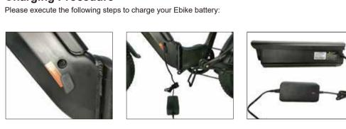
1. Ensure the bike is off. 2. Remove the rubber cover on the charging port. 3. Plug the charger into the battery's charging port, BEFORE PLUGGING CHARGER INTO POWER
