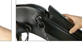
**Step1**: Ensure the bike is turned off. Align the key port with the appropriate "locked" position by inserting the key into the key port, and then rotating to align the key with the "unlock" icons, and the battery will pop up.
