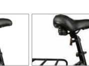
Step 6. Open the clamp under the seat post, set it to a height which fit for the rider then close the clamp to secure the seat in place.
