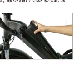
battery weighs 9.45 lbs and should be handled with care.
