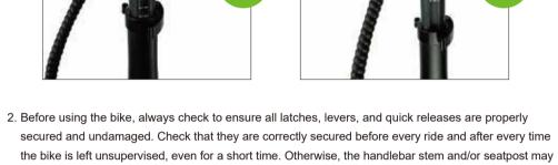
the bike is left unsupervised, even for a short time. Otherwise, the handlebar stem and/or seatpost may come loose and can result in loss of control, damage to the bike, property, serious injury, and/or death. Adjusting the Suspension Fork
