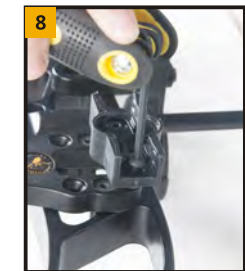
Install the quiver base on the bow sight (install the screw in holes of the last line on the bow sight) like in the picture 8
