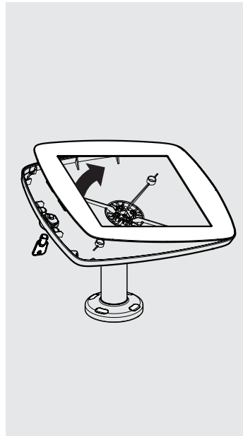
6 Unlock & remove the Faceplate from the Bouncepad Case.
