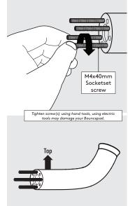
Locate and screw the Socket screws into the Branch as shown.
