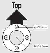
Using the Mount washer, **A1** mark the drill hole locations as shown.
