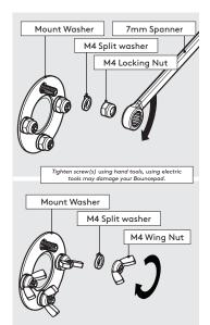
Secure the arm to the surface. Locking Nuts offer higher security.
