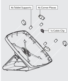
Install the Tablet Setup Kit. Each kit is specific per tablet device and Bouncepad Case.
