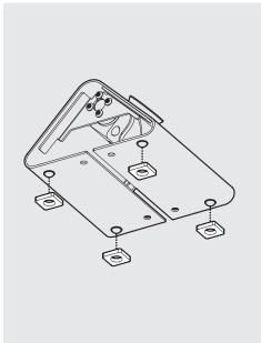
If wishing to slide your Flip across your mounting surface, apply the supplied Felt Feet as shown.
