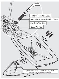
Attach the Bouncepad Case to the Flip. Take care to ensure correct & full thread engagement.
