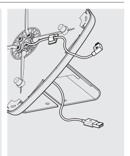
Route the Bouncepad Cable through the Case and Flip - securing it with the Cable Clip.
