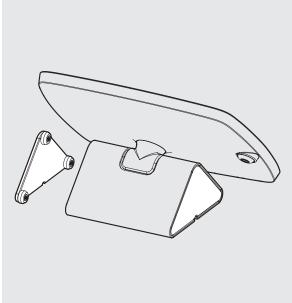
Locate the Flip End Plates onto the Flip Base.
