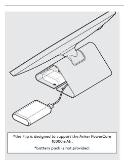
If installing a battery pack, connect the tablet cable and locate the pack into the Flip.
