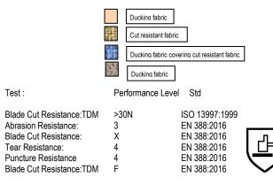
Test Results - The levels of performance are uniform except in the cutter apron.
