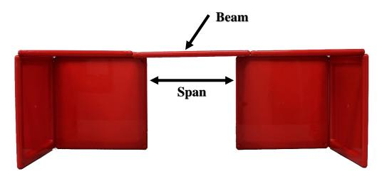
The **span** shown above is supported at both ends. The **span** shown below is supported at one end, and in the middle. This creates a condition called a **cantilever**. A **cantilever** is a beam anchored at only one end. **Cantilever** construction allows for overhanging structures without external bracing.
