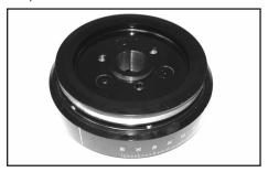
Out of the box damper is set up for use on a 427 or other FE engines with one pulley. For 1967 and earlier engines with more than one pulley, see above.
