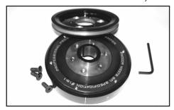
For 1968 and later FE engines with more than one pulley, remove the Professional Products pulley using an Allen style hexagonal wrench.
