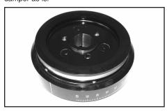
Out of the box damper is set up for use on a 427 or other FE engines with one pulley. For 1967 and earlier engines with more than one pulley, see above.
