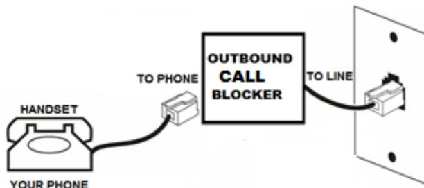
**PROGRAMING:** After installing it, lift off the handset connected to the PHONE port of the device and use the dial-pad to program your device as shown below.
