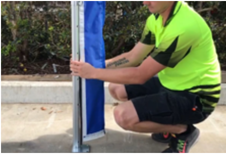
5. Press the Leg Rubber Inserts into the tracking on the Lower Leg of the tent. Repeat on other side.
