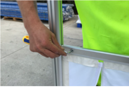
8. Using the supplied tool, tighten the bolt lightly. Repeat on other side. Adjust the Half Wall Bar as need to be level and in desired position, tighten bolts to secure.
