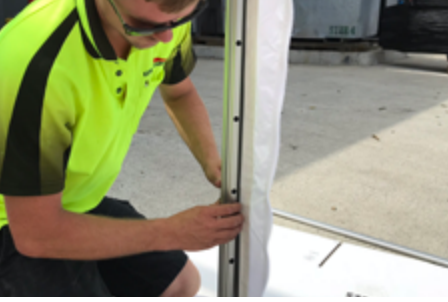
4. Press the Leg Rubber Inserts into the tracking on the Lower Leg of the Canopy. Repeat on other side.
