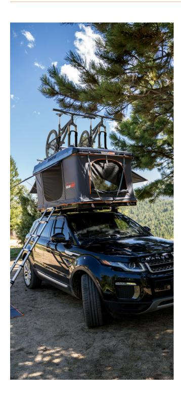
Roofnests are engineered to be mounted to two crossbars that are at least 30 inches apart. Platform racks can be used, but are not necessary and in some cases make installation trickier.
