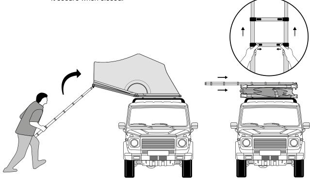
STEP 4 | Secure the two straps between the tent frame and the ladder crossbar, put the cover on the tent with the Roofnest Logos facing to the front and back of your vehicle.
