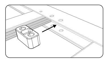
STEP 3 | Place the Ladder Mounts over the holes.
