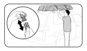
STEP 2 | Release the strap on the ladder, then extend the ladder.
