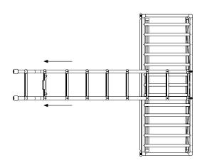
STEP 3 | Hold the bottom of the ladder as a lever to press down and unfold the tent, then adjust the length of the ladder as needed.
