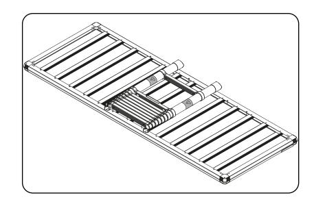
STEP 8 | Insert 1 M8x1.25mmx15mm Button Head Hex Drive and 1 M8 Locknut connecting the ladder to the ladder mount.
