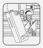
To correct this, hold the latch up so the connecting plate is level.
