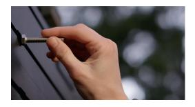
Accessory Channels on all four sides of the top and bottom shell allow you to attach anything to your Condor Overland like lights, awnings, showers, etc (weight limit per channel is 50 lbs and the more spread out the attachments the better).
