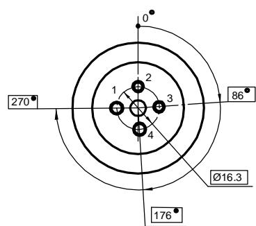
Electrode -to - lead connection diagram
