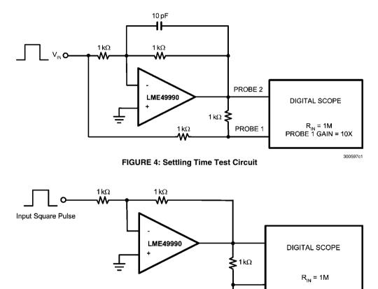
FIGURE 5: Slew Rate Test Circuit
