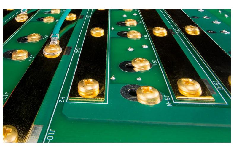
The P20 is all new in design and construction. Instead of wires to route power, there are aerospace-grade pure-copper, 1/4" thick gold-plated buss bars handling all current paths.
