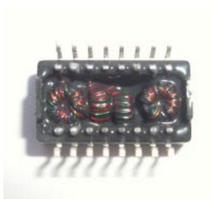
The actual transformers are tiny toroid's, inside an SMD package.
