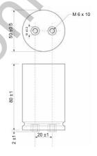
Specifications casing 3: Bucket: aluminum bucket, unshrunken UL 94-V0 Terminals: internal screw thread M6 x 10 Weight: approx. 215g
