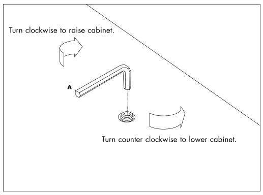
The other two adjustable leveler glides are located in the rear center of the bottom shelf. Use **Allen Wrench (A)** to adjust.
