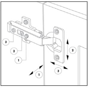
Adjustments may be made to Novia's door hinges with the use of the Phillips head screwdriver. Each hinge assembly has three (3) adjustment screws:
