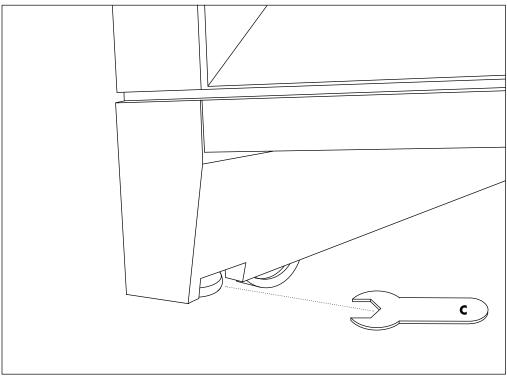
Two of the four leveler glides are accessible near the bottom of the side panels using the **Leveler Wrench (C)**.
