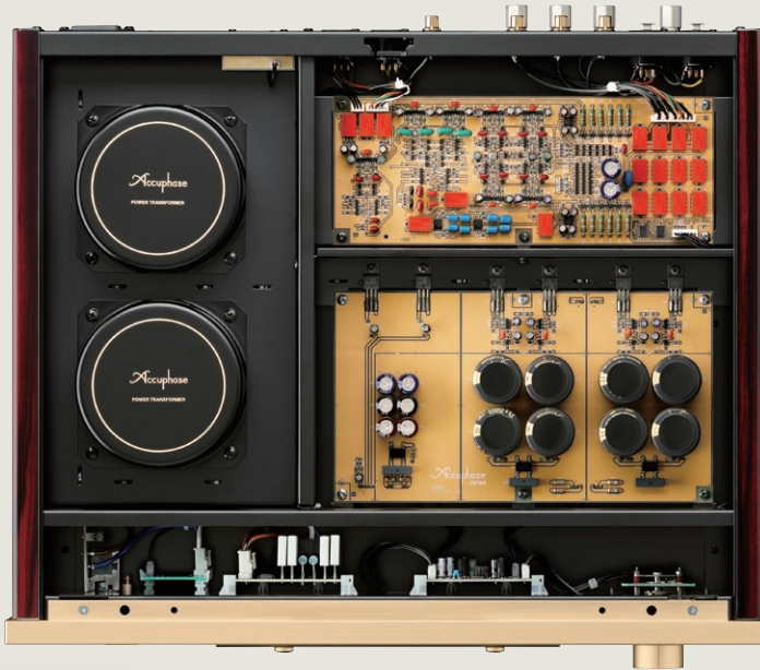
Internal layout realizes full mono construction to prevent mutual interference between channels
