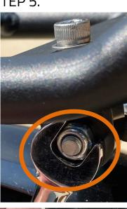
Step 4- Take one of the black bolts and pass thru the hole on the bottom of the rear rack and align with the treaded portion on the bottom of the bike frame-Tighten but keep slight loose. Now do the same on the other side. You will need the 4mm Allen wrench
