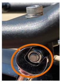
Step7- Go OVER all areas on your rack and TIGHTEN and SECURE all BOLTS and NUTS. You should be checking 6 BOLTS and 2 NUTS.
