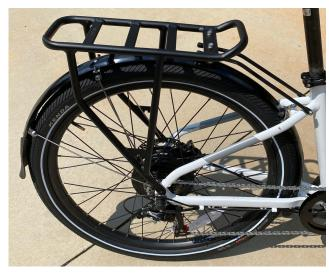
**Step 3-** Loosen but do not completely remove the nuts and bolts on the top of your rack. FOUR (4) positions. Once loosen you should be able to move the bars freely. For the top- USE your DENAGO folding tool 5mm Allen wrench. For under the rack, you will need a 10mm or adjustable wrench. In loosing these 4 areas this will allow you to adjust the rack in STEP 5.
