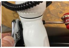
**Step 3-** Secure the bolt using your Denago Multi Tool and an adjustable wrench. Keep bolt loose until you add the fender rods.
