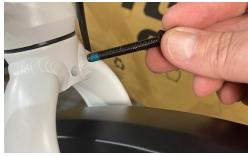
**Step 2-** Take long bolt and larger washer and nut. Add washer to bolt and feed thru the bolt hole on the front fork and thru the fender tab. Connect the bolt.
