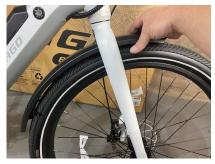
**Step 1-** Grab Front Fender and feed from back of wheel forward. Keeping TOP fender tap on back of fork.
