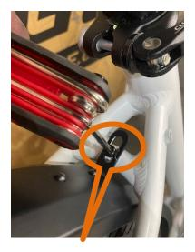
**REAR FENDER Step 1-** Grab Rear Fender and feed from back of wheel forward. Keeping TOP fender tap on back of frame. Take allen bolt and small washer and thread bolt thru fender tab and thread into frame bracket. Do not tighten YET
