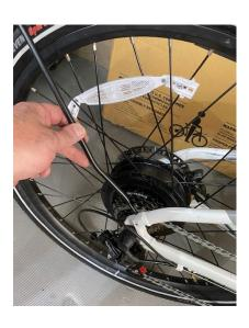
**Step 20-** Take longer rack rods. Place BOWED out section to bottom of frame. Take small allen bolts and connect top of rod to rear fender. No not tighten
