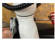
**Step 6-** Check alignment and secure and tighten fork bolt on top fender tab
