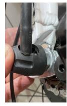
**Step 18-** Reconnect motor cable. Ensure pins are all straight- Align both ARROWS on each side
