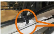
**Step 19-** Zip tie motor cable to frame bracket.
