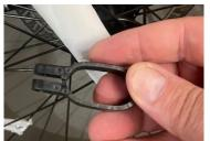
**Step 5-** Take fork brackets and apply to forks with bolt tab facing to the back of the frame. Insert allen bolt slide in rod into center of bracket and insert nut into the space on bracket
