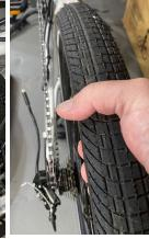
Step 12- You will some good finesse and force pull rear wheel up and back. You might need to pull rear derailleur back to help removing rear wheel
