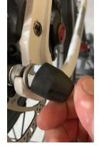
**Step 17-** Apply axel caps on the rear axel nuts. Press firmly
