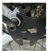
**Step 16-** With axel position in place and inside position axel stopper washer in place secure and tighten the rear wheel with the Denago wrench.
