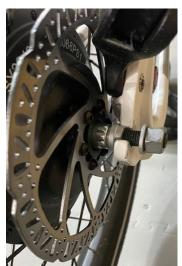
You are now prepared to check alignment and secure axel nuts
