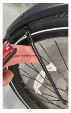
**Step 4-** Take shorter rods along with 2 of the small allen bolts. Secure rod to back section of fender but do not tighten YET.
