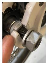
**Step 8-** On the NON-DRIVE Side (NO GEARS) Remove the black cap. Make sure to set aside for replacement **Step 9-** Use Denago Wrench and LOOSEN Axel nut NOTE- Axel is slotted and with a unique washer stopper
