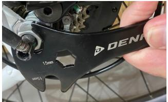
**Step 10-** On the DRIVE Side (With GEARS) Remove the black cap. This threads thru the motor cable. Make sure to set aside for replacement
