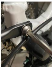
**Step 21-** Remove the 2 silver bolts by the seat. Take this and connect the bottom portion of the fender rods to the screw hole on the bottom of the frame. Connect and secure but do not tighten.
