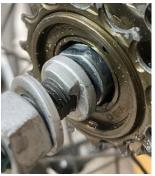
The Axel Stopper washer is positioned on the iside of the frame and on the outside is a flat washer and the axel nut.
