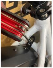
Step 22- Align and secure all three sections. Bottom of Fender Rod Bolts. Top of road bolts and center bracket. ALGIN and SECURE and TIGHTEN
