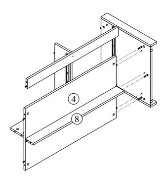
Attach the Front Support Panel (7), Back Support Panel (6), Bottom and Plinth Panel (4) & (8) to Left Panel (2) by screwdriver (not provided).
